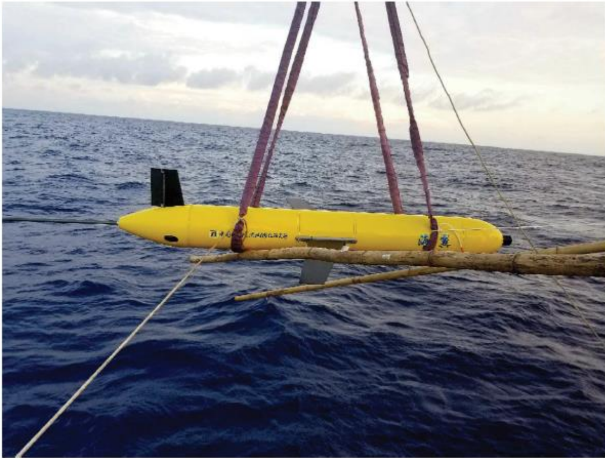
Photograph of an acoustic Sea-Wing underwater glider
