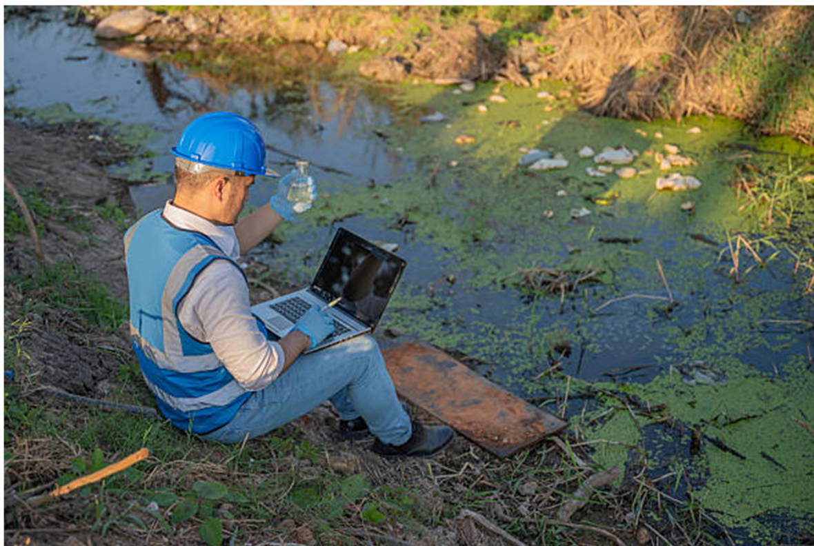
Figure 3: Field monitoring and water sampling. An environmental engineer logs real-time data while analyzing a water sample from a stagnant, eutrophic water body. Source: Pexels
