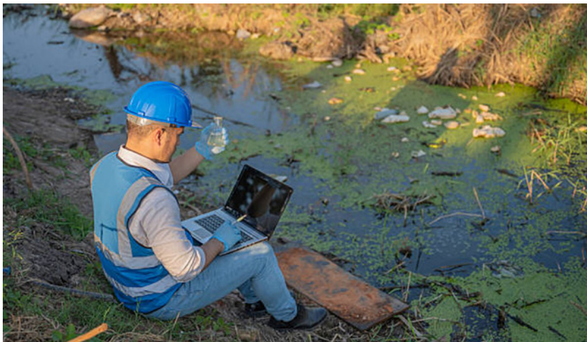
Figure 3: Field monitoring and water sampling. An environmental engineer logs real-time data while analyzing a water sample from a stagnant, eutrophic water body. Source: Pexels
